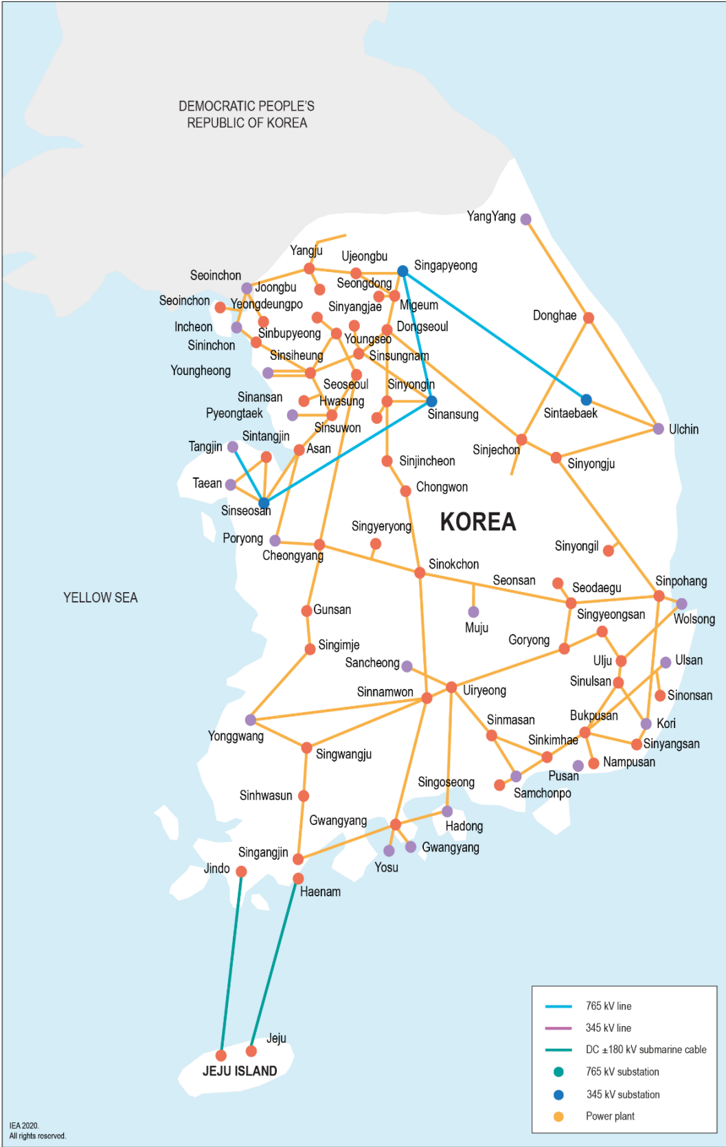
Figure 7.8 Korea's transmission grid
