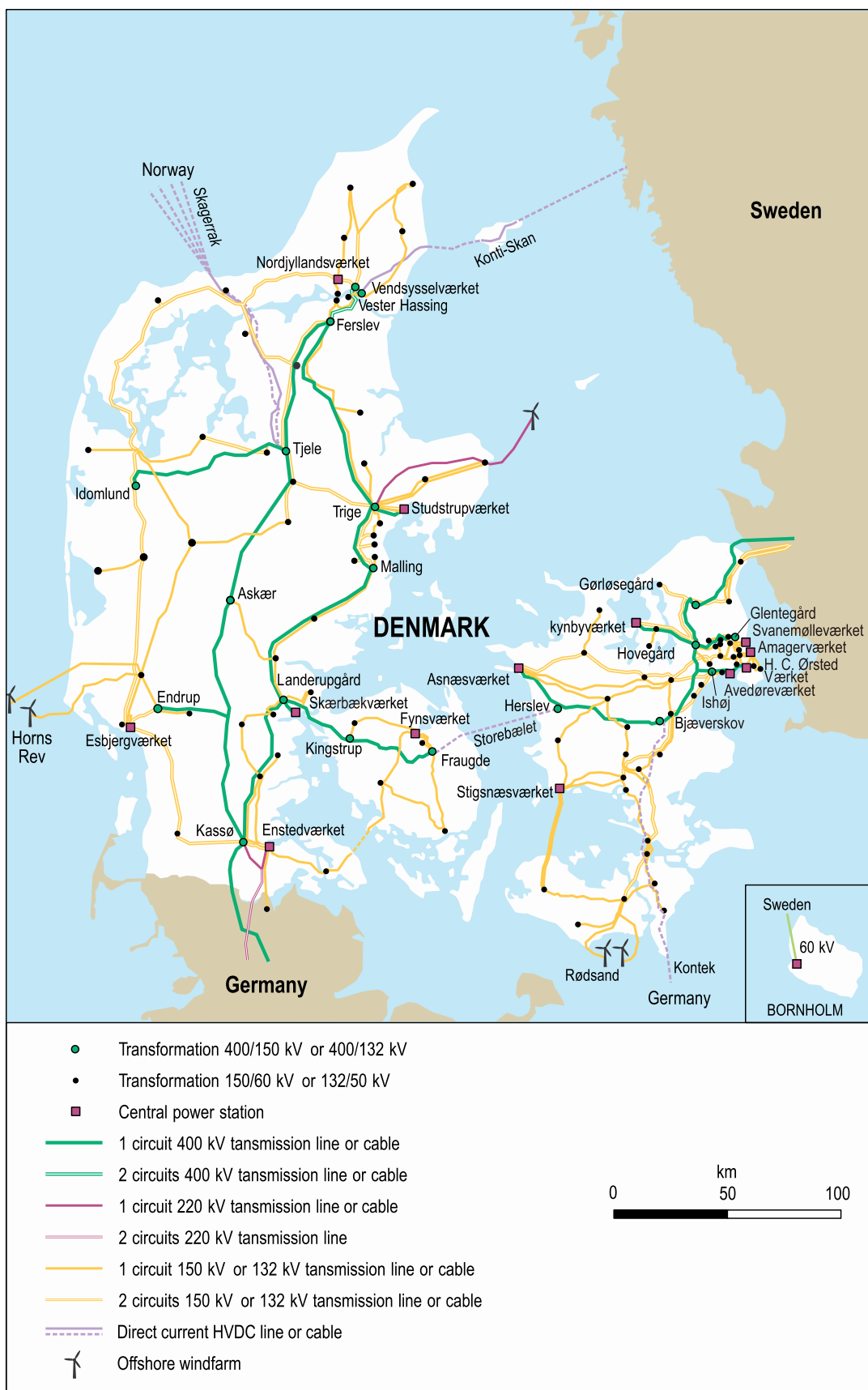
Figure 5.7 The Danish electricity transmission system
